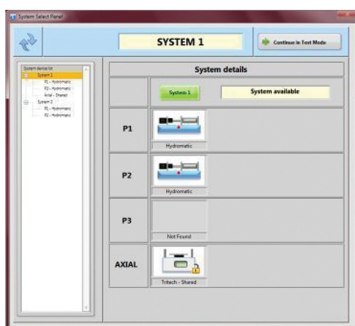
System selected panel showing two triaxial systems are available, with one shared Trittech compression frame
